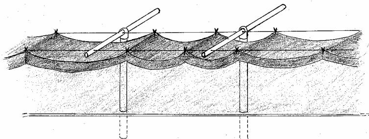
Figure 13.14. Modified drift fence for catching treefrogs after Murphy (1993)
